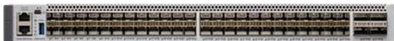
Figure 4. C9500-24Y4C: Cisco Catalyst 9500 Series high-performance switch with 24x 25 Gigabit Ethernet + 4x 100G Uplink
