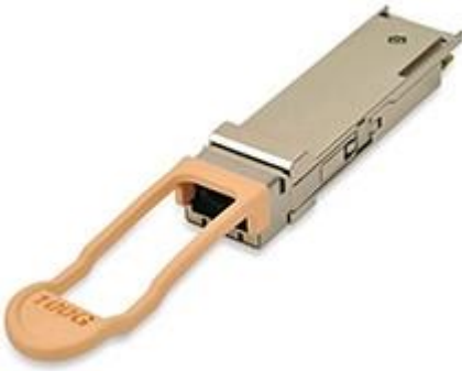
Figure 5: QSFP28 optical transceiver module that use MPO connectors
