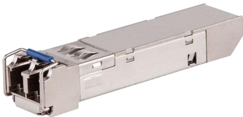
Figure 15: Gigabit or 100-Megabit SFP optical transceiver module
