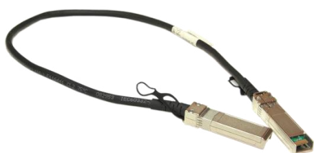
Figure 13: SFP+ DAC cable
